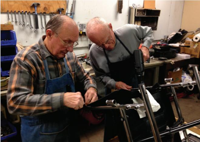
*Jim Damer and George Telle dismantle a wheelchair to clean and check and replace bad parts with good before lubrication and reassembly.*
